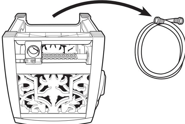
2. With unit in overturned position and when facing the front of unit, ensure that hose guide is located in far left location and that locking lever is in closed position.
