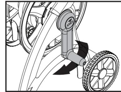
REEL HOSE IN BY TURNING CRANK IN CLOCKWISE DIRECTION AND GUIDING HOSE EVENLY ONTO REEL WITH FREE HAND.
