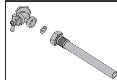
ENSURE A RUBBER WASHER IS INSIDE EACH FITTING OF THE LEADER HOSE AND YOUR GARDEN HOSE TO AVOID LEAKS BEFORE CONNECTING TO SPIGOT AND HOSE REEL WATER SYSTEM.
