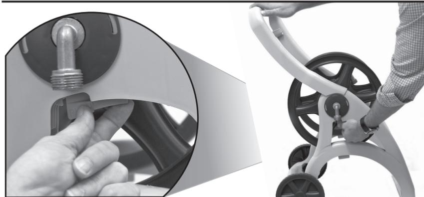
TO LOWER HANDLE, PRESS THE PUSH BUTTON IN THE MIDDLE OF THE FRAME WHILE SIMULTANEOUSLY PUSHING THE HANDLE DOWN. TIP: USE YOUR INDEX FINGER TO PULL ON TAB OPPOSITE OF THE PUSH BUTTON TO MAKE THIS EASIER. REPEAT ON THE OTHER SIDE AND THEN PUSH THE HANDLE ALL THE WAY DOWN.
