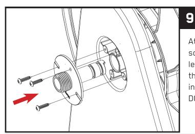
Attach the outer water system piece using the three
