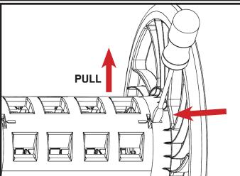
Insert a small flat head screwdriver into the slot as shown. Apply force to the latch toward the center of the unit as indicated by the arrow. By simultaneously pulling on the hub half, the latch can be disengaged as seen below. Repeat this for all four latches on a hub half.
