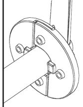
Interlock the two retainer halves you removed earlier around the new aluminum water system. Place them as shown in order to hold the water system in place.
